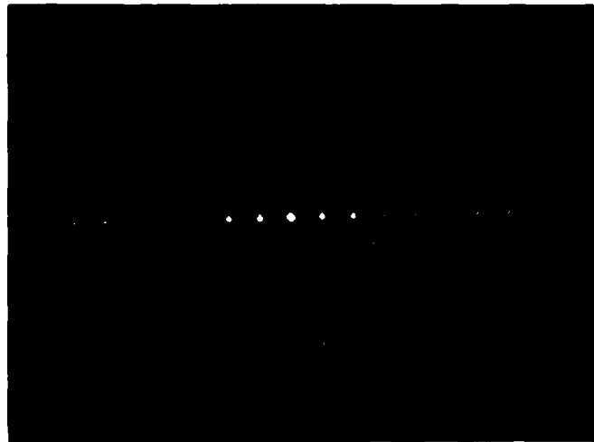
Figure 12. The Fourier transform spatial spectrum of the one-dimensional screen as shown in Figure 11.
