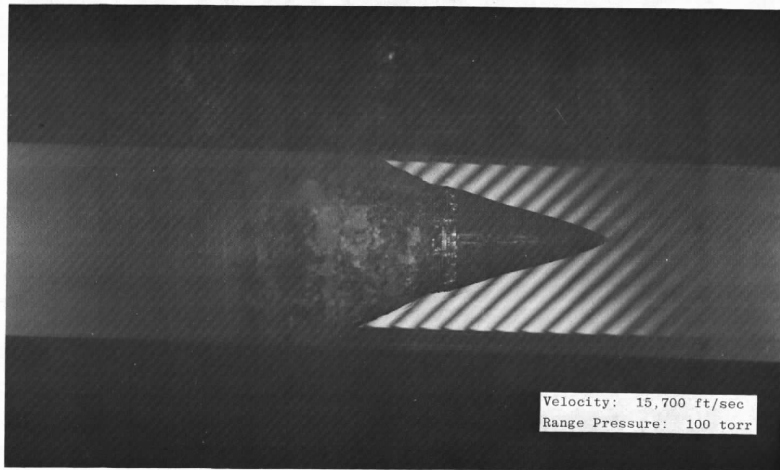
Figure 9. Laser photograph of gas jet model: 30-Å-wide bandpass filter used in recording camera.
