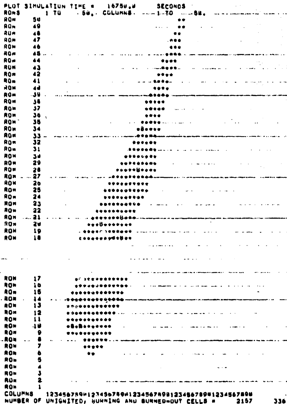
Figure 6-8(f). Cell state map for small area fire, ambient wind = 20 m/s.
