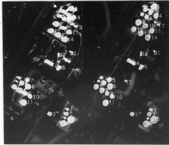
Figure 8. Low altitude model image matching without group information Left: view 1, Right: view 2
