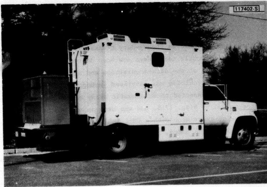
Fig. V-1. Mobile node with acoustically quieted engine/generator mounted at rear.
