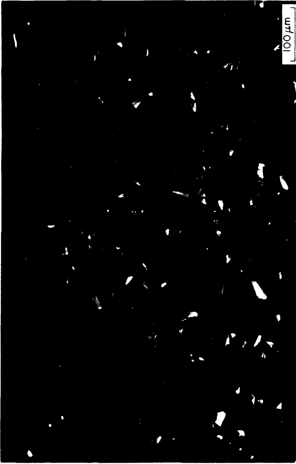
Figure 6. Enlarged Fracture Surface of Glass-10 vol SiC, Showing the Interaction of the Crack Front with the Particle obstacle.
