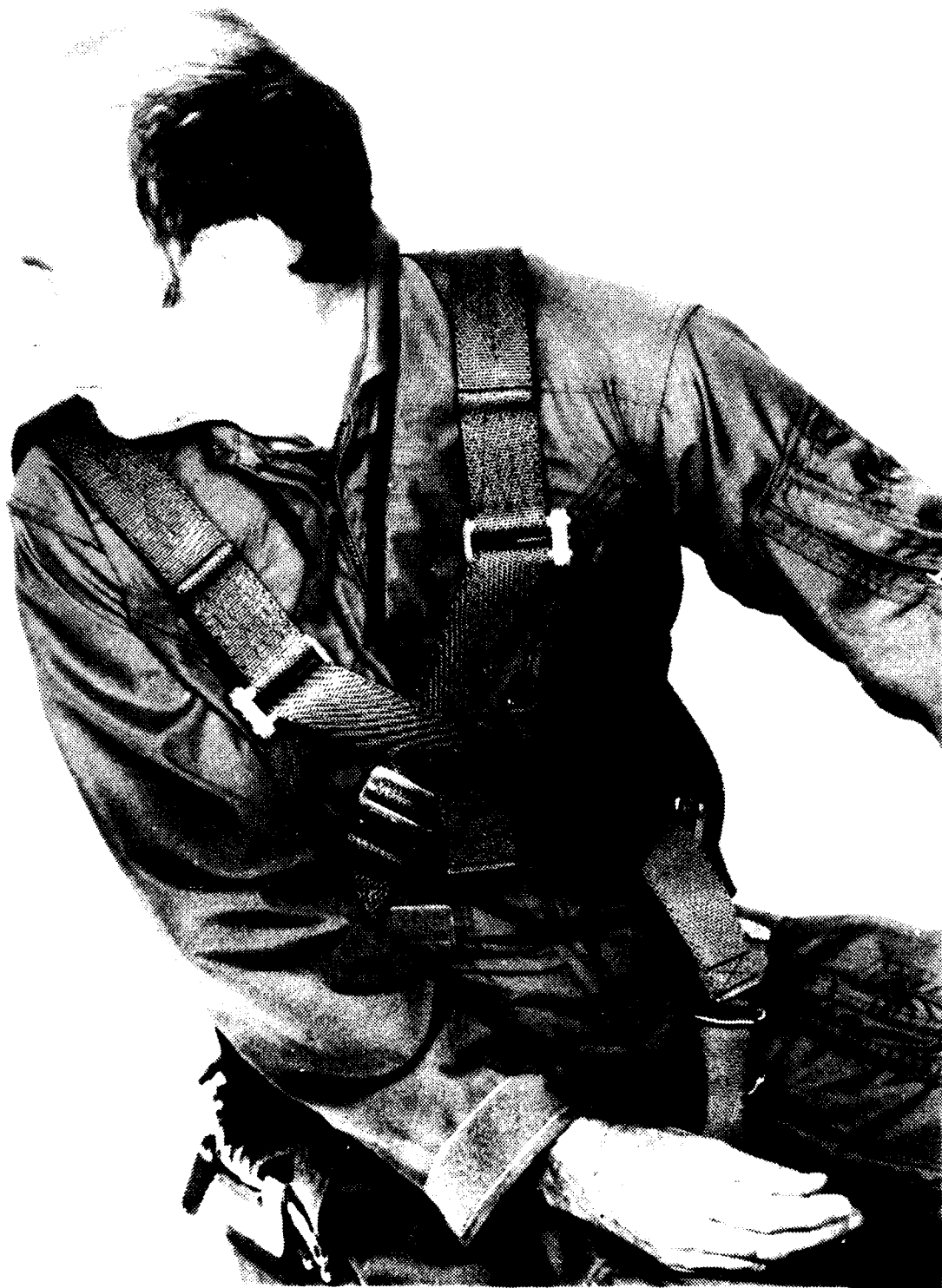
Figure 6. XV MOD 1 With Roller Fitting Which Allows Rotation
