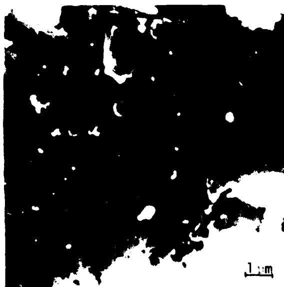
(b) Microfracture details within right-hand sector of subsurface zone in (a); microcracks are oriented parallel to P.
