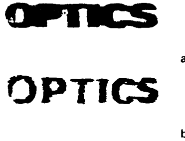
Fig. 4a and b. Photographic image deblurring with encoded extended incoherent source. (a) Input blurred object and (b) deblurred image.
