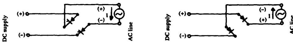
Figure A-2. Two paths of power flow from wind-generated DC source to AC lines.
