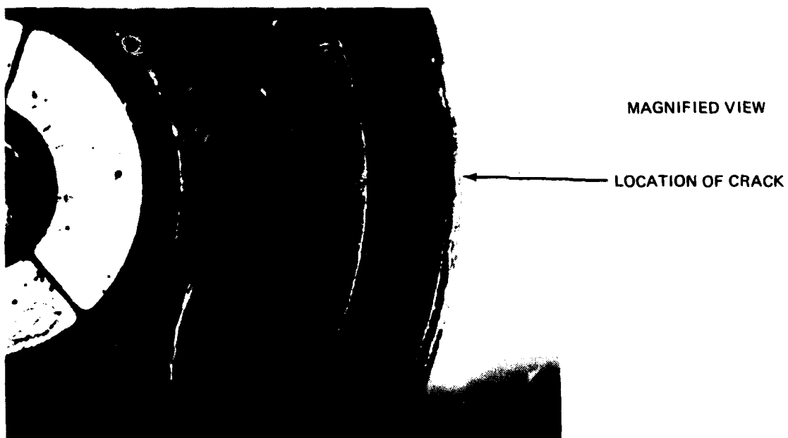
Figure 3 - SCR Silicon Sub-assembly Showing Radial Crack
