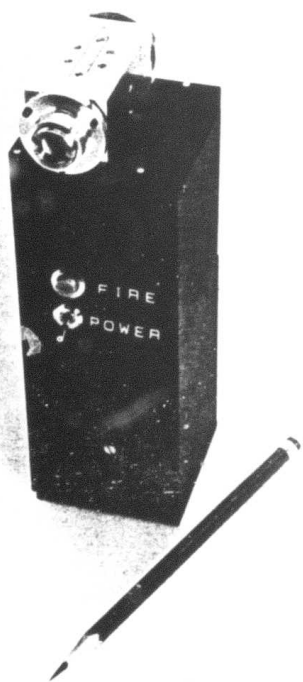
Figure 21. Hand held laser setup (SHH) and its laser head showing pump cavity (coated with Kodak white reflectance coating 6080) flashlamp, NPP rod, KSF filter, and Q-switch.
