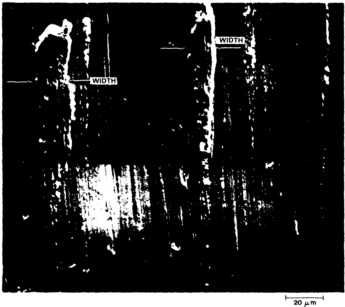
Figure 41 - Copper Transfer to Inconel Counterface Showing That the Transfer Patch Widths in Later Stage Wear Roughly Correspond to the Widths of Deformed Regions Shown in Figure 40
