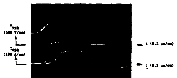
Fig. 8. RSR voltage and current when functioning in a typical pulse modulator circuit
