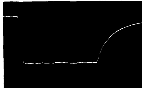
Fig. 6 Model 3 Driver. Klystron Pulse. Vertical 10 kV/div Horizontal 0.5 \mu s/div
