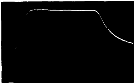
Fig. 5 Model 2 Driver. Klystron Pulse (shown inverted). Vertical 10 kV/div Horizontal 0.5 \mu s/div
