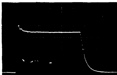
Fig. 9 Model 3 Driver. Switch Tube Grid Voltage. Vertical 200 V/div Horizontal 0.5 \mu s/div
