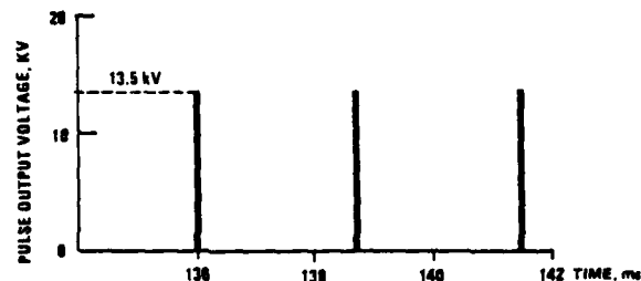
FIGURE 5B. ECAP PREDICTED OUTPUT PULSE AMPLITUDE AT CONSTANT PRF OF 360 PPS
