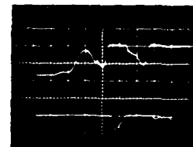
Figure 9. Oscillations In End-Of-Line Clipper, Load Initially Open, Shorted Near End Of Pulse
