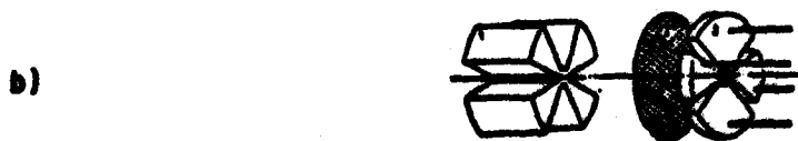
Elements of the velocity-spread analyzer: 1) iris with sectoral slits; 2) antidynatron grid; 3) sectioned collector.
