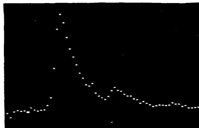
Figure 6. Photographs of the N_2 CARS signal obtained in room air and a flame environment using collinear geometry. (a) room air, (b) a rich CH_4/O_2 flame without shielding from air contributions, and (c) the same flame as in (b) except shields were used to eliminate room air contributions.
