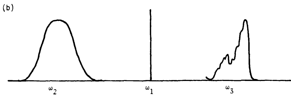
Figure 1. (a) Representative energy level diagram where \omega_1 and \omega_2 are laser frequencies, \omega_3 is the CARS signal produced and \omega_{v,R} is an allowed molecular vibrational or rotational energy spacing. (b) Representative frequency spectrum when using broadband laser radiation centered at \omega_2 .
