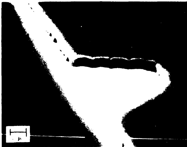
Figure 2-25. Improvement Due to Increase in Contrast Factor Is Readily Apparent for PMIPK Resist
