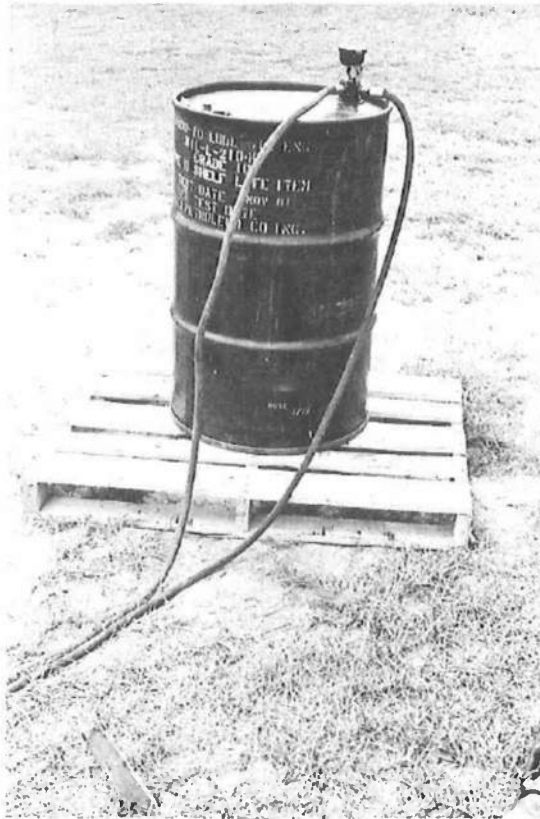
Figure 67. Fuel Fill-Vent Assembly Installed
