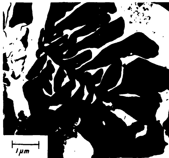
Fig. 5--Extraction replica of grain boundary carbides from astroloy given H-3 heat treatment.
