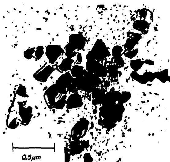
Fig. 6--Extraction replica of grain boundary carbides from astroloy given H-4 heat treatment.
