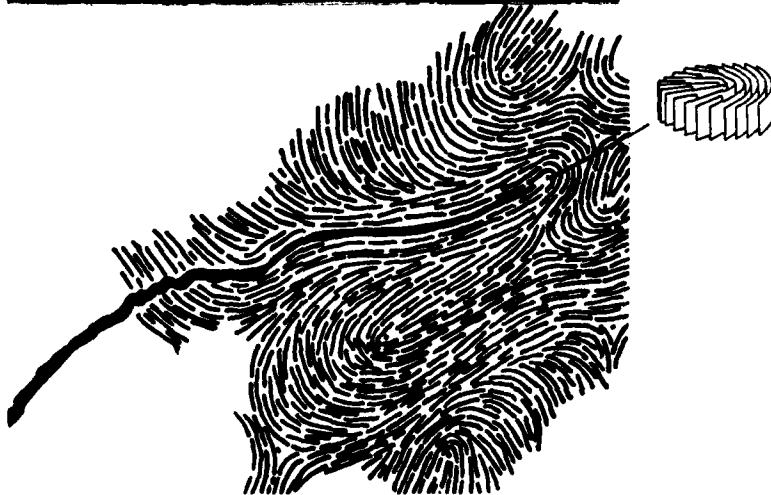
Figure 13. Crack blunting at disclination of strength S = +1/2 .
