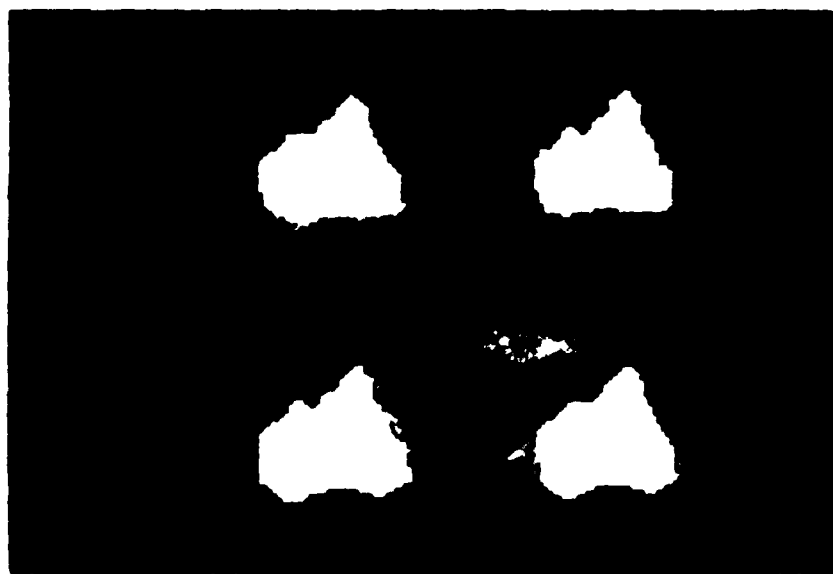
Plate 1. Portion of Record 21 of Westinghouse LLR Tape. Slice program output using Method 1. Upper pictures represent output using iterated 3 by 3 mean filter and 3/5 rule. Bottom pictures represent 5/9 rule and 13/25 rule.
