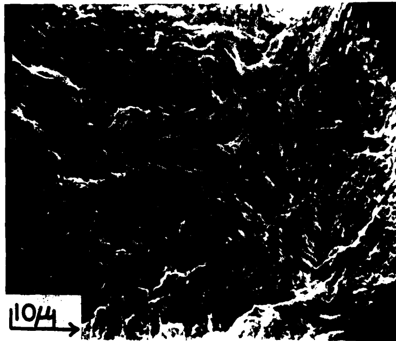
Figure 28. Scanning electron micrograph of the fatigue fracture surfaces of the dual phase IAA of HY80 steel.
