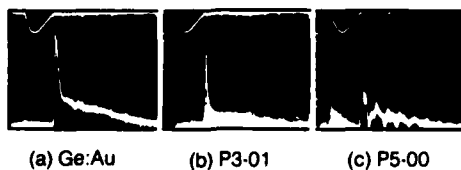
Figure 6. Pulse shapes with different detectors: 500 ns per div., 1000 pps, He:CO 2 :N 2 4:2:1, 280 Torr, 20 Torr \ell /s; mirror reflectivity, R = 0.94, minimum delay adjustment. (Note piezoelectric ringing of pyroelectric P3-01 and P5-00 detectors.) Discharge current waveform is shown in top traces.
