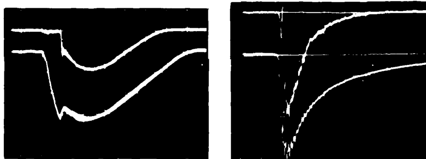
Figure 3. Current and voltage waveforms. Upper traces: 10 A and 200 ns per div. Lower traces: 500 V and 200 ns per div. Right picture: 30- \mu H coil shorted.
