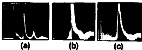
Figure 7. Pulse shapes and jitter: (a) maximum power adjustment, same parameters as for figure 6, Ge:Au detector. (b) 100 ns per div., P5-00 detector, 1000 pps; 1-s exposure indicates pulse jitter. (c) 30- \mu H coil in pulse circuit shorted out. 100 ns per div., P5-00 detector, 1000 pps; 1-s exposure indicates pulse jitter. Same discharge current waveform as shown in figure 3. Other parameters in (b) and (c) are same as for figure 6. Ringing preceding laser pulse in (c) is due to unwanted coupling from discharge circuit.
