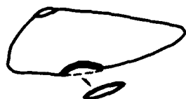
B. REMOVAL OF "HALF MOON" SPALL.
