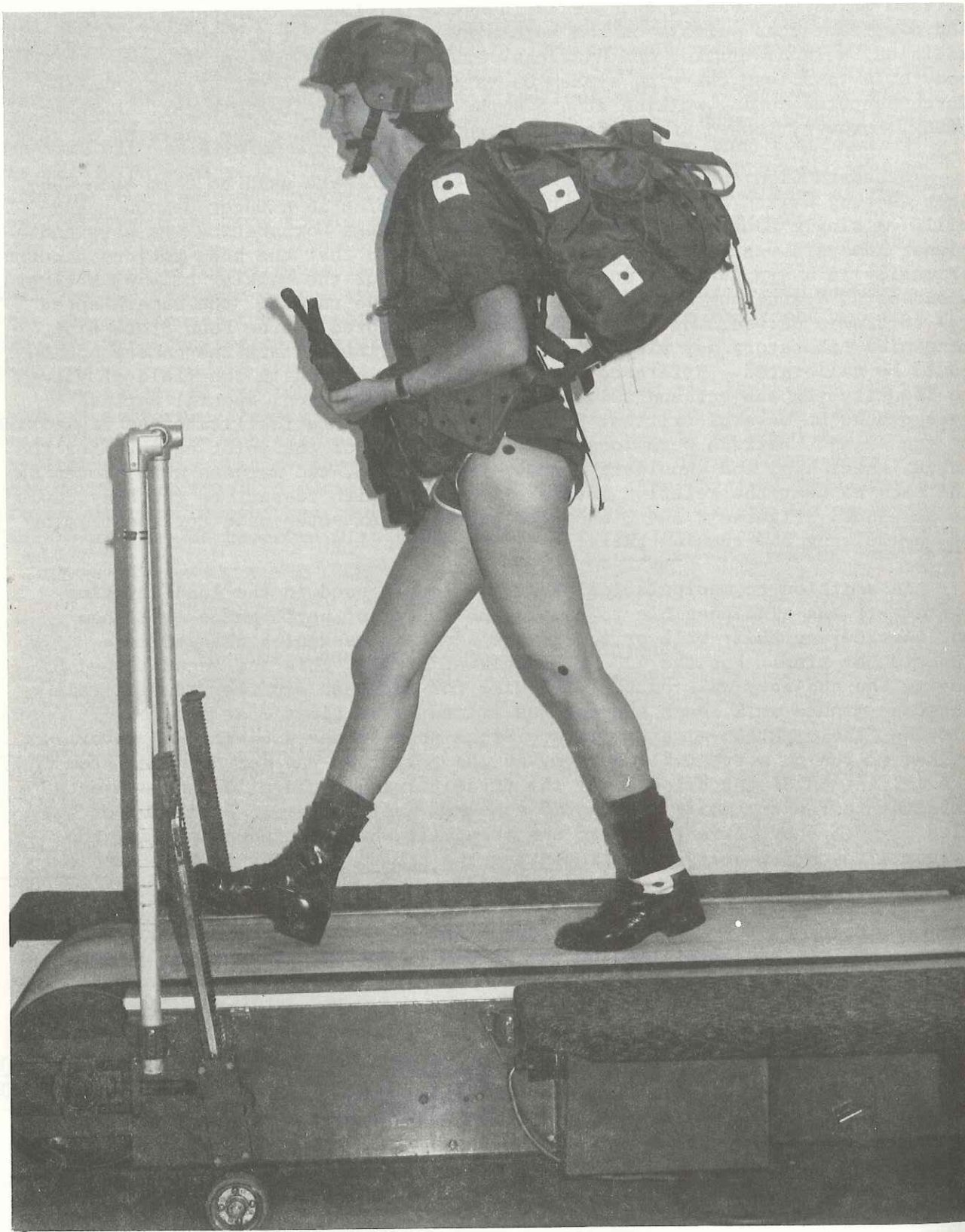
Figure 2. Subject performing treadmill walking. Note the markers placed on the body and pack to facilitate analysis of the cine films.
