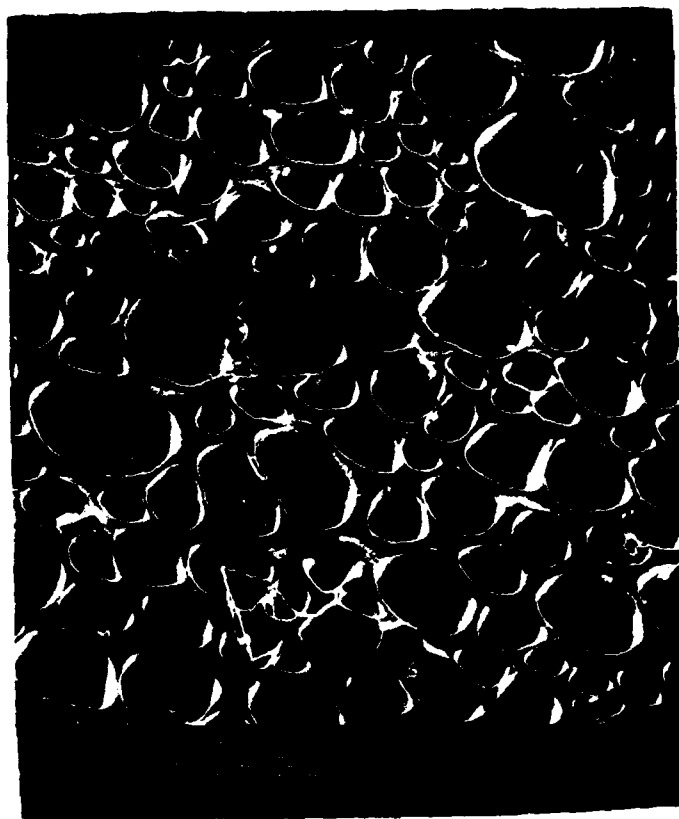
Figure 6. Scanning electron micrograph of polyurethane-modified acrylic latex deposited at 75 V. Film thickness = 16 mil. Magnification = 100 X.
