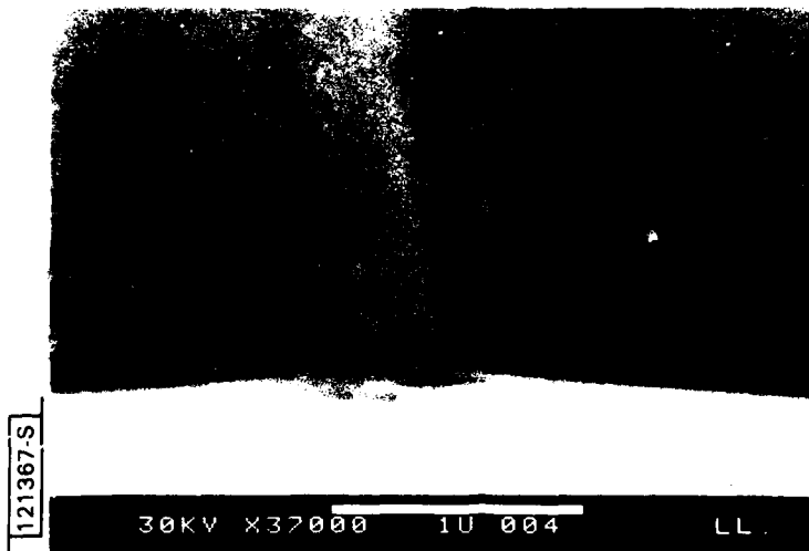
Fig. 4-7. Submicrometer gap etched in GaAs with SF 6 at 0.47 W/cm 2 power density.
