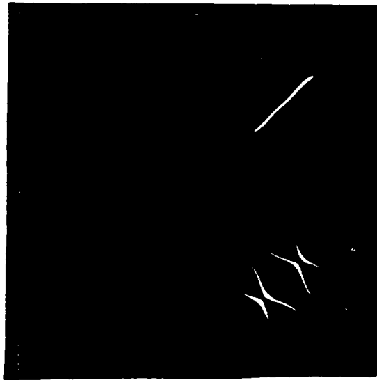
Figure 5 : Top row, left; detected targets using causal model. Top row, right; detected targets using semicausal model. Bottom row; images shown in top row are now shown on dB scale. Causal model has better resolution than FFT processing, but has false alarms. In general, semicausal model spectra are found to be more accurate.
