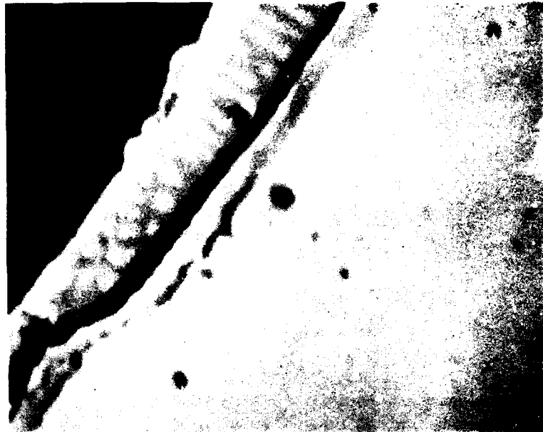
Fig. C.3. Electron image of surface slag formed on electrode tip droplet in Ar + 2 vol% O 2 (2000X).
