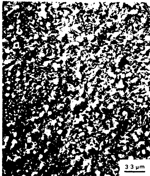
Figure 34. Heat-treated material; H2+A2+T1/≤44 μm screen. Kalling's etch. SEM.
