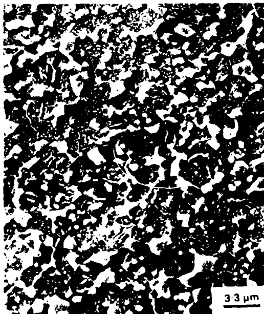
Figure 12. HIPed (H2) 250-840 \mu\text{m} screen; Kalling's etch. SEM.
