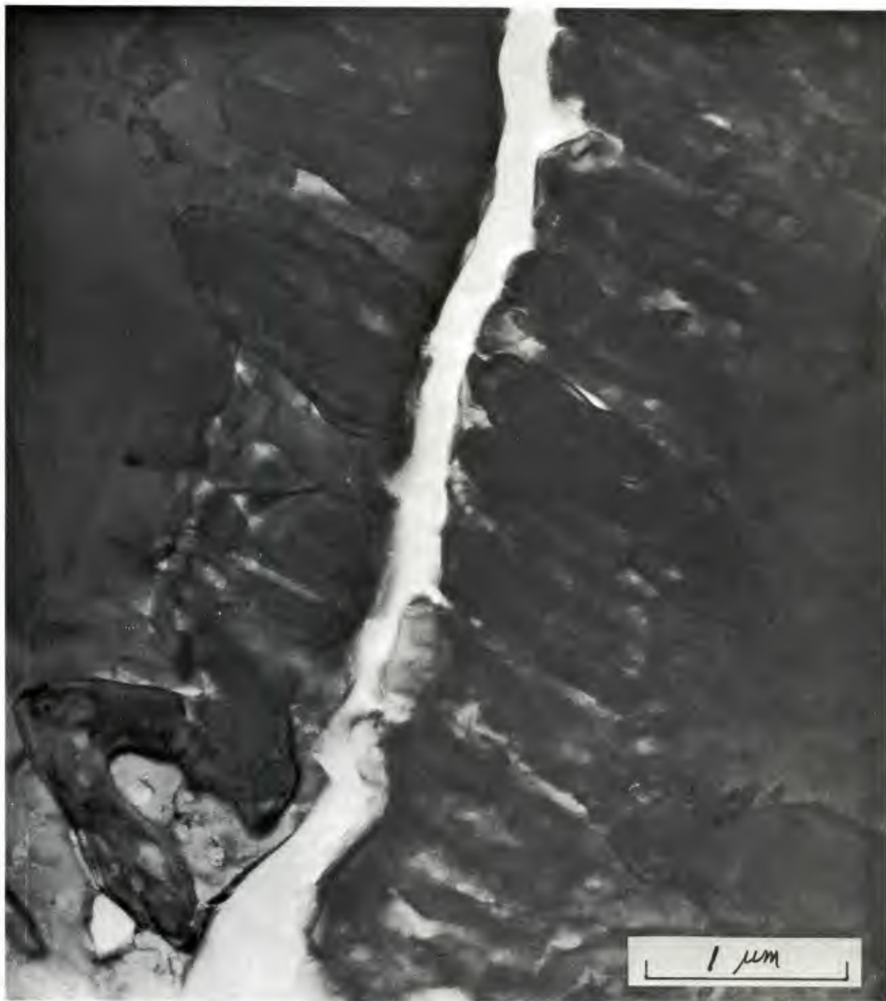
FIGURE 20 Columnar grain growth on adjacent, previously melted rack (or boundary) faces in central region of cylinder of dynamically compacted alumina, TEM. In this locale, energy density during passage of the shock wave was sufficiently high to cause brief localized surface melting ( T_m 2050°C) to a depth of 1-2 \mu m , as evidenced by columnar grain growth (normal to the melt surface) during subsequent cooling (Yust 1980)
