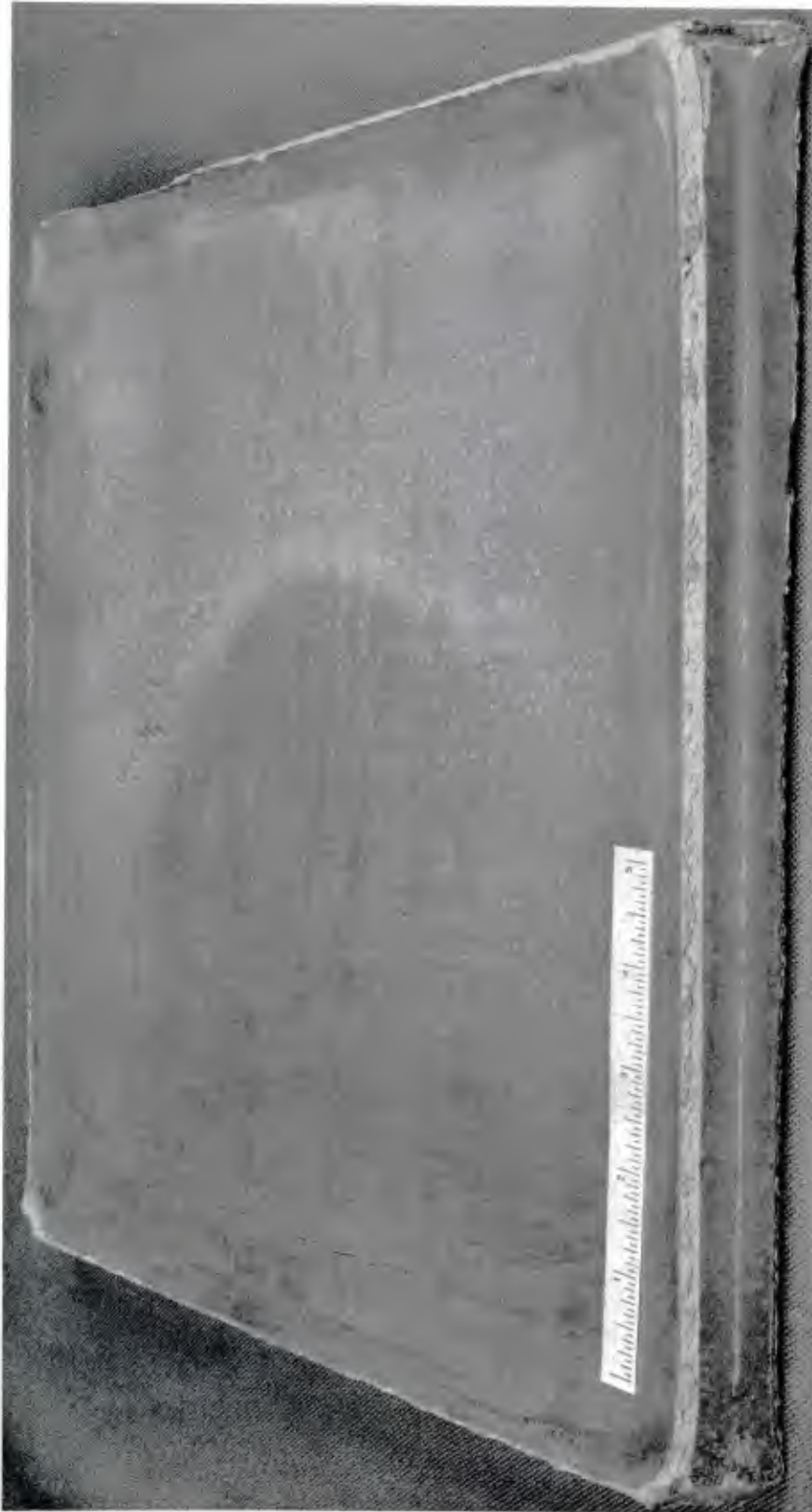
FIGURE 32 Explosively compacted T.D. nickel plate with overall size of 1x14x14 inches (Linse 1981)
