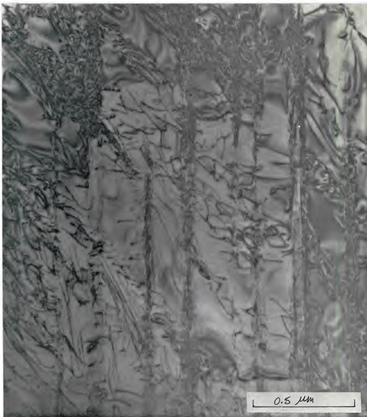
FIGURE 21 Detail of individual dislocations and dislocation arrays within a grain at the half-radial position in a cylinder of dynamically compacted alumina, TEM. Shock-induced strain clearly is present in the form of dislocations. The operative slip systems were not limited to the basal plane, which is oriented in the vertical direction (Yust 1980)
