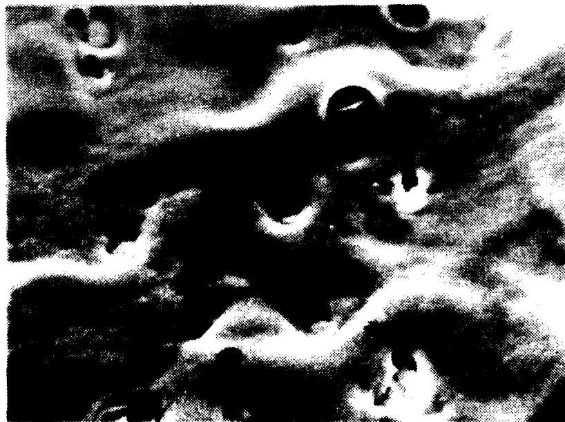
Figure 31. Unpolished SS-304 after Irradiation with 400 MW/cm 2 , SEM 2350X
