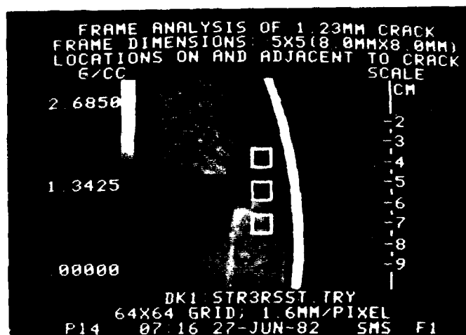
FIGURE 23. Tomogram of 1.23 mm crack in 470 mm phantom, with size (5 pixels x 5 pixels = 8.0 mm x 8.0 mm) and location of density analysis frame indicated (adjacent to and on the crack).
