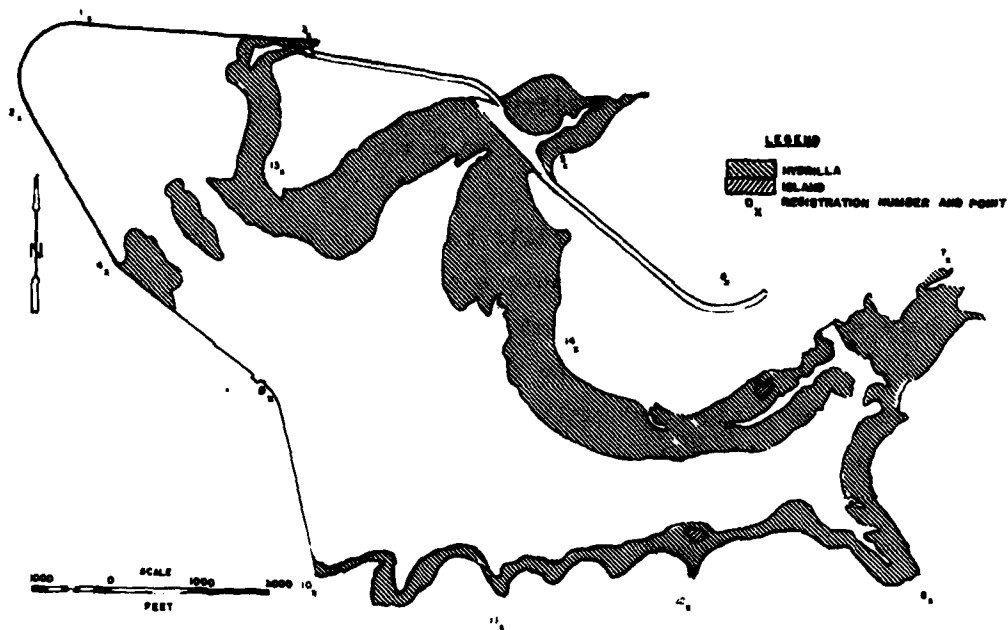
Figure 2. Areal coverage of hydrilla and locations of control (registration) points, Lewis Creek Reservoir, Texas, as mapped on overlays of the 1:6000-scale (nominal) color imagery
