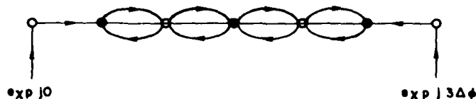
Fig. 14 — One-dimensional CAM lattice. Empty circles denote amplifier/limiter modules terminated by an antenna; filled circles denote modules with nonradiating terminations. This figure is equivalent to Fig. 2.
