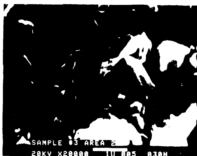
Fig. 5.26 S.E.M. Micrographs of Polyurethane Coating of Type "B" on E Glass Epoxy Substrate After Exposure to 200 gr of Sand Impacted at Impingement Angle of 30 Degrees. (A) General View x 540. (B) Enlargement of A x 2100. (C) High Magnification of Eroded Area Showing the Embedment of Sand Particles x 2000. (D) Very High Magnification of Eroded Area x 20,000.
