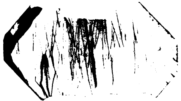
Figure 2. 11\bar{2}0 Topograph of \langle 10\bar{1}0 \rangle Slice of High Purity Quartz Grown on a High Purity Seed
