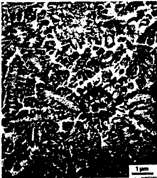
Figure 3. As-atomized T15 powder, \leq 37 \mu\text{m} ; Kalling's etch. SEM.
