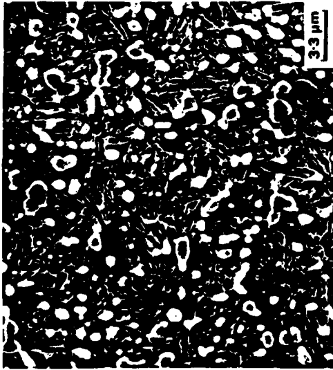
Figure 33. Heat-treated material; H2 + A1/250-840 \mu\text{m} screen (T15). Kallling's etch. SEM.
