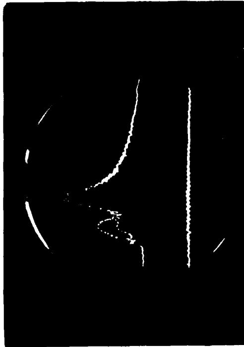
Upper trace: APD#4 100 mV/div (enhanced) 100 ns/div
