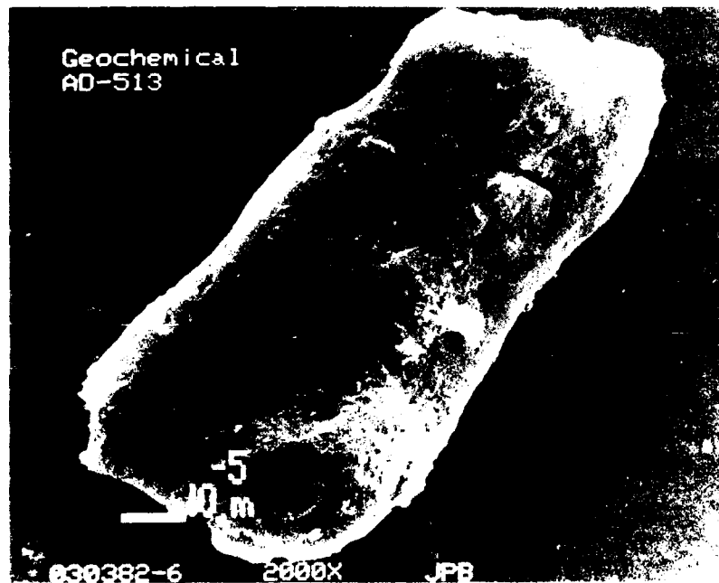
Fig. 2. Scanning electron micrograph of quartz grain after HF acid treatment. The pitted, grooved surface is not as apparent with this grain as it is in many such grains. Fragments of glass still remain on the right side of the grain.
