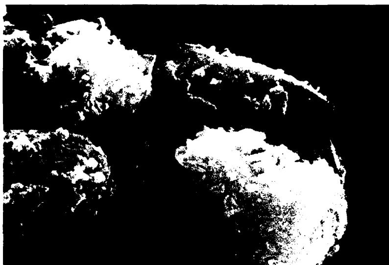
Fig. 5. Scanning electron micrograph 020582-1 of tiny wedge-shaped crystals believed to be titanite, X9000. Crystals are about 5 \mu\text{m} .
