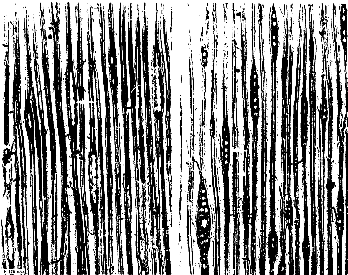
Figure 2.--Photomicrographs of tangential surface of pine showing wood rays opened by mold infection (arrow at left) and normal rays with cells intact (arrow at right); wood-invading bacteria affect ray cells similarly.
