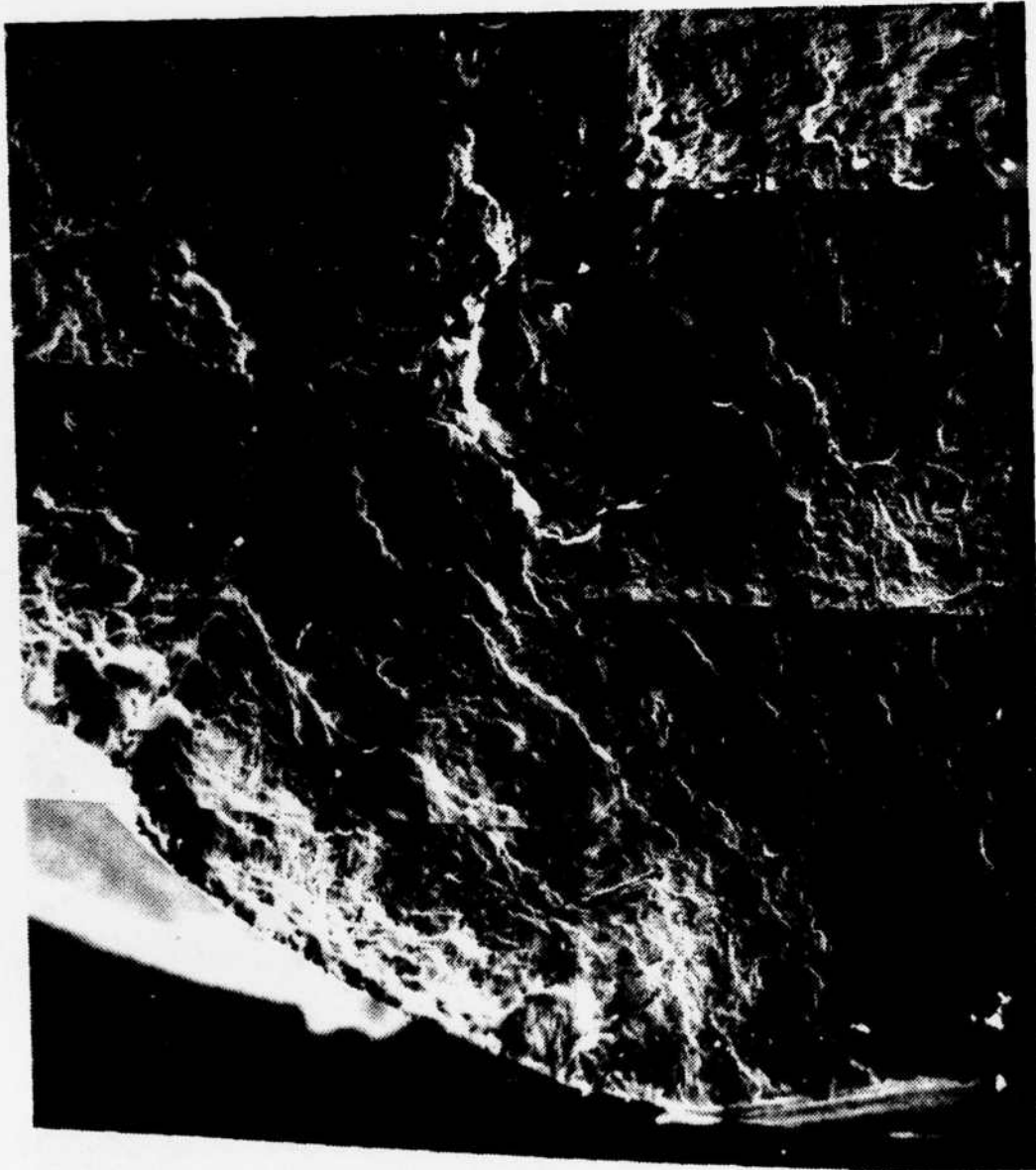
Figure 25. 1/2 Fracture Surface of Normalized and Tempered Material Subjected to 1/2 Hour Dwell Periods and Continuous Cycling in Vacuum . Specimen No. 12 (28x)
