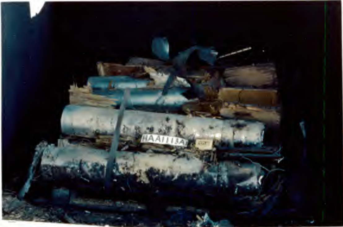
Figure 28. Results from a simulated pallet fire test using fire-retardant treated packaging
