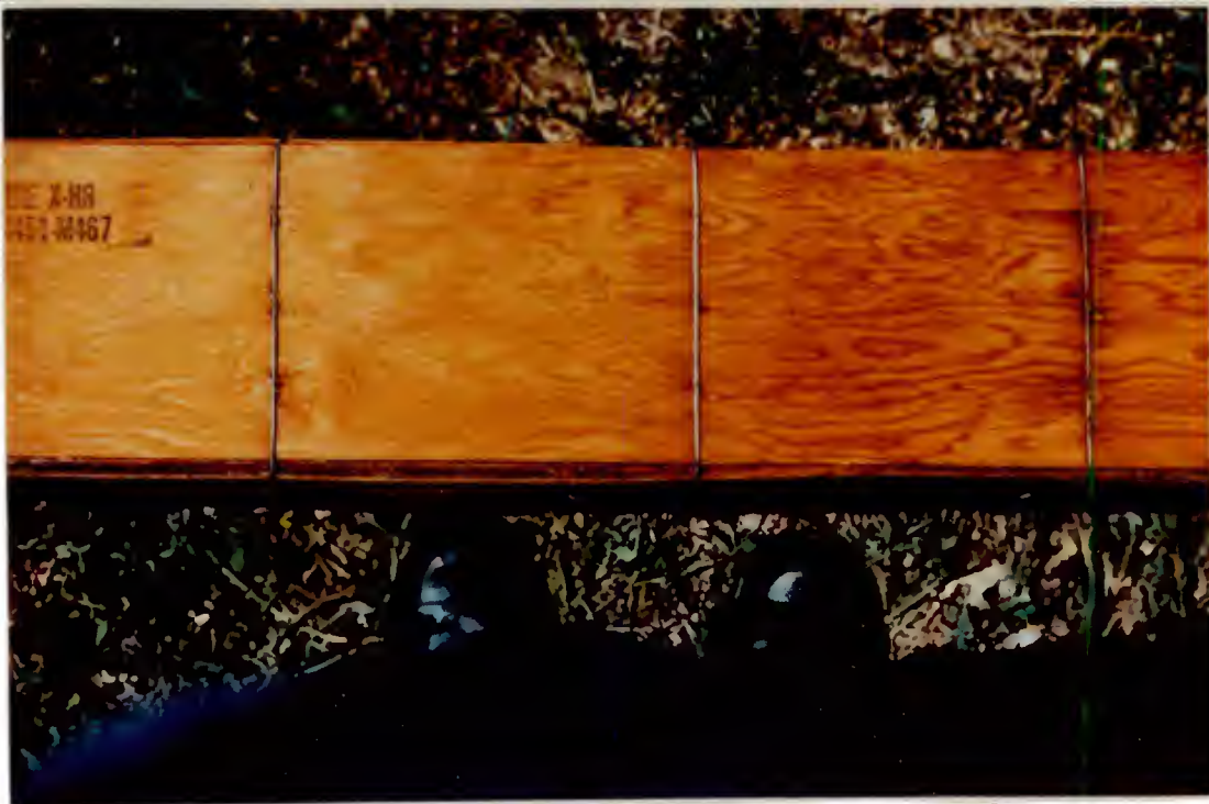
Figure 25. Fire-retardant-treated box after a 3-month exposure
