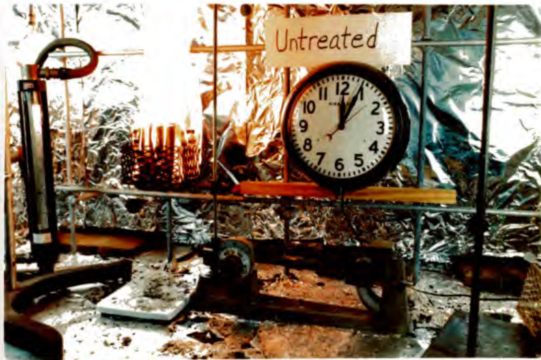
Figure 8. Crib test performed on untreated wood--68 seconds after burner shutoff
