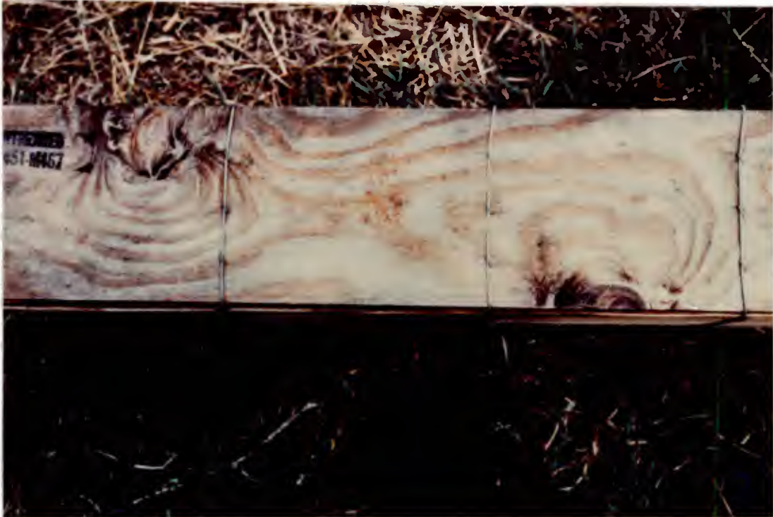
Figure 24. Untreated box after a 3-month exposure
