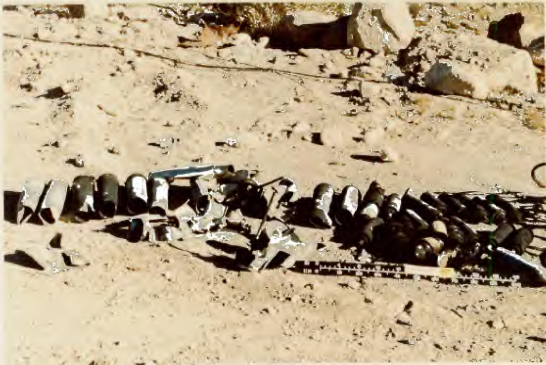
Figure 27. Debris remaining after a simulated pallet fire test using untreated packaging
