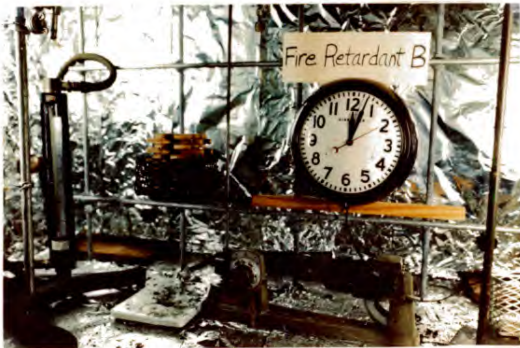
Figure 10. Crib test performed on fire-retardant treated wood--10 seconds after burner shutoff
