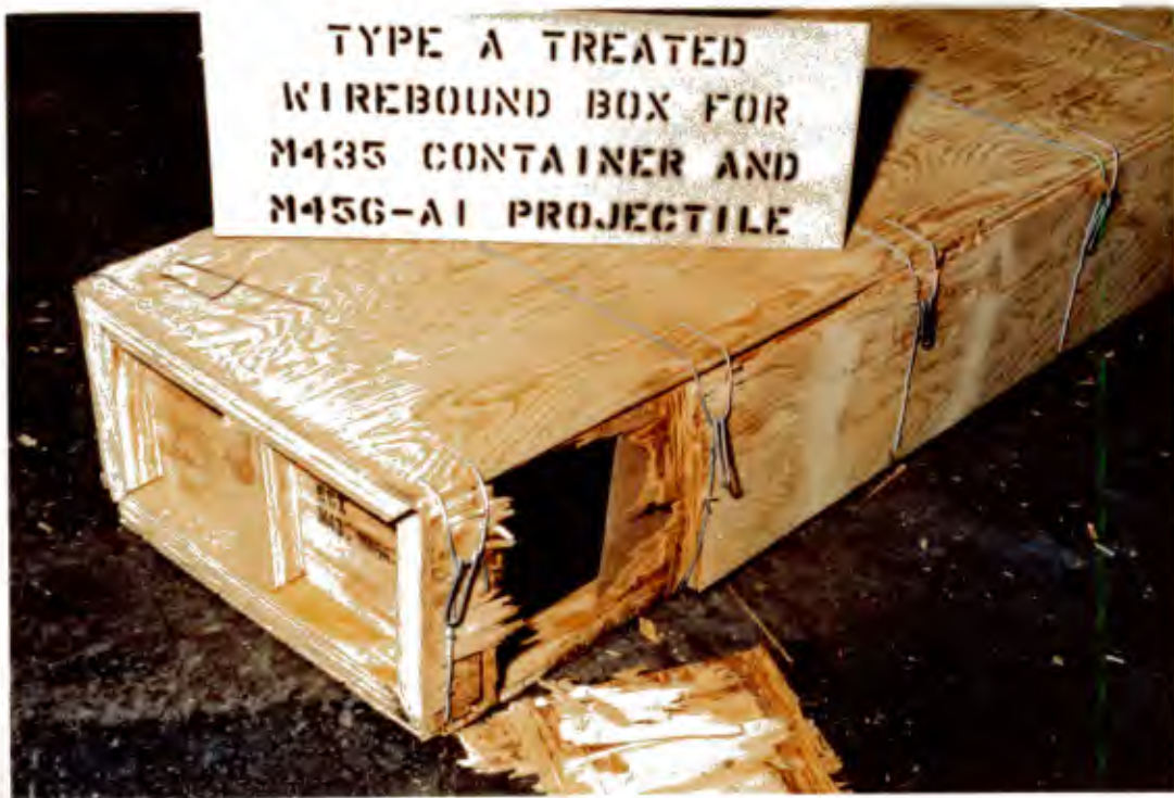
Figure 21. Fire-retardant-treated box after completion of the drop-test series
