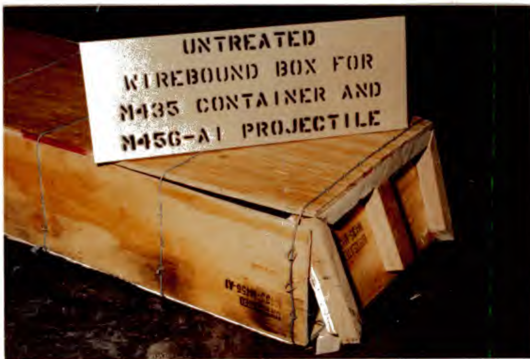
Figure 23. Untreated box after completion of the drop-test series
