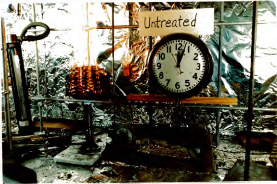
Figure 7. Crib test performed on untreated wood--5 seconds before burner shutoff
