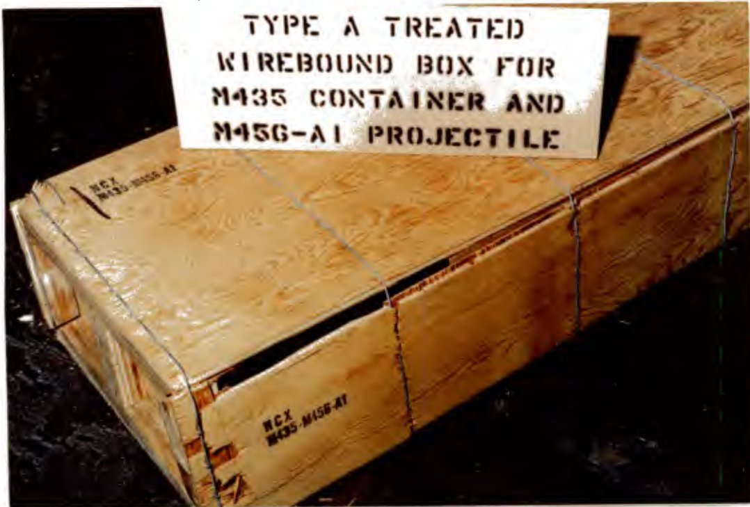
Figure 20. Progression of damage to a fire-retardant-treated box during the drop-test series
