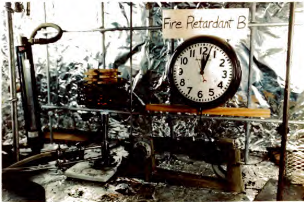
Figure 9. Crib test performed on fire-retardant treated wood--5 seconds before burner shutoff
