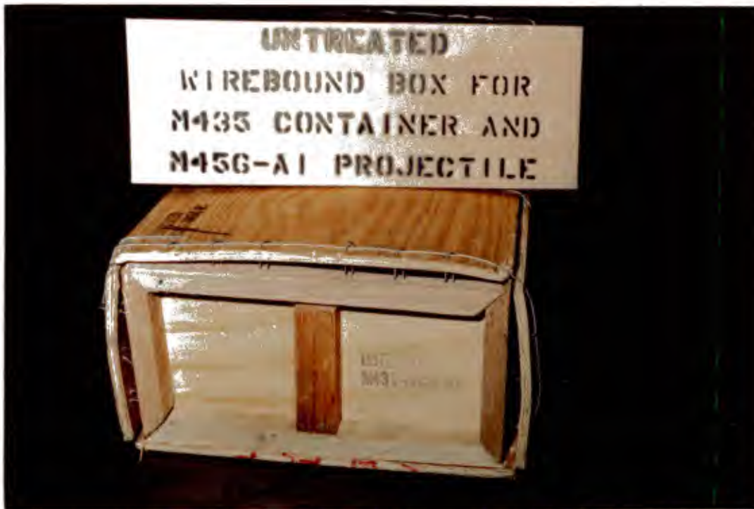
Figure 22. Progression of damage to an untreated box during the drop-test series
