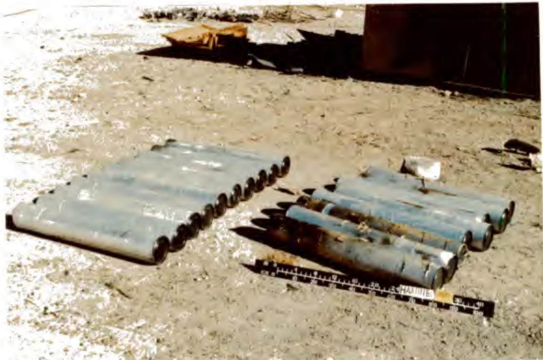
Figure 29. Intact rounds remaining after a simulated pallet fire test using fire-retardant treated packaging
