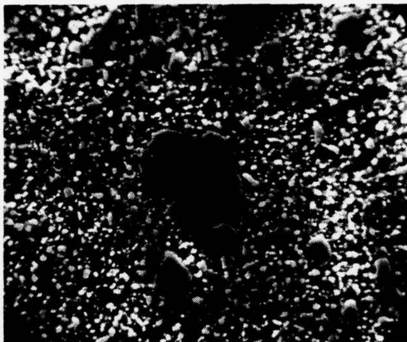
Fig. 19 As-received material showing residual carbides on a background of temper carbides. Magnification 2400X
