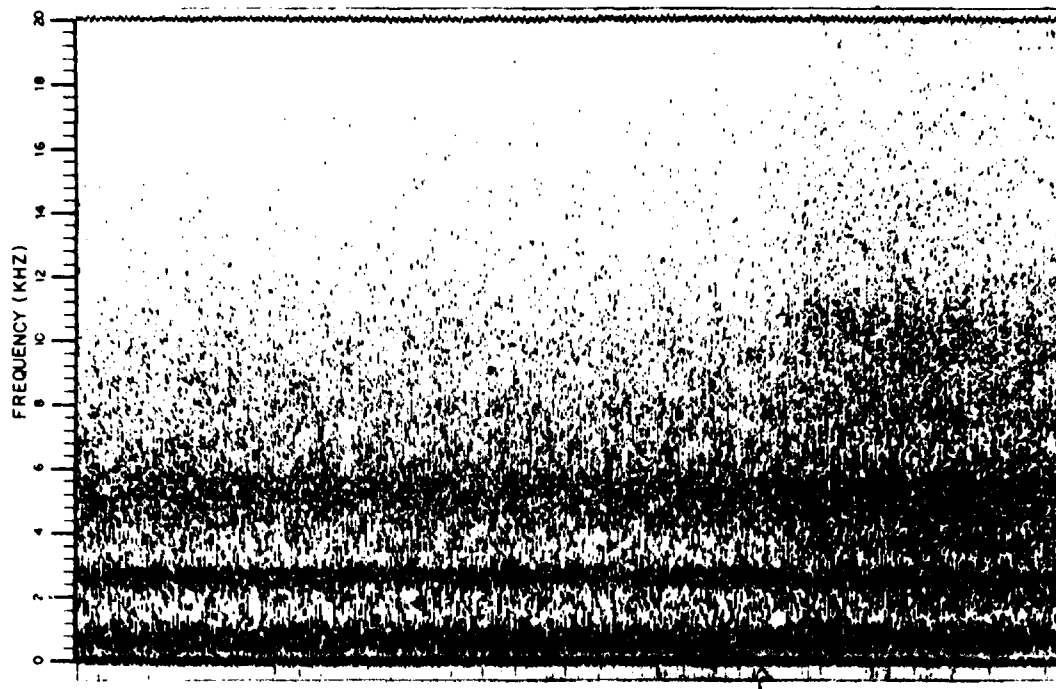
Figure C-28. Microphone No. 5 Spectrum Analysis. Analysis Bandwidth is 0 to 20 kHz.
