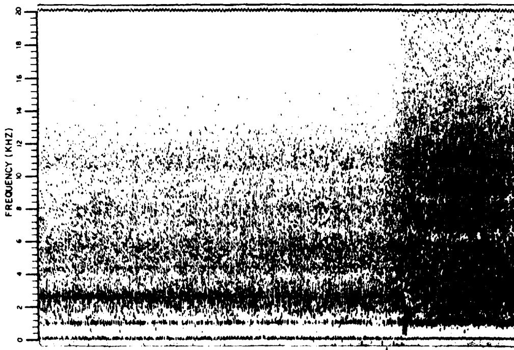
Figure C-24. Microphone No. 2 Spectrum Analysis. Analysis Bandwidth is 0 to 20 kHz.
