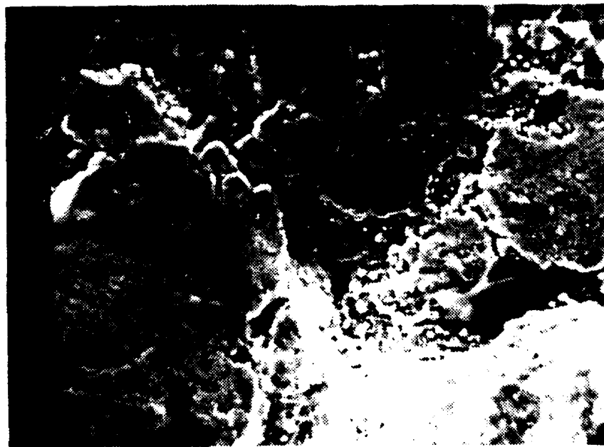
Figure B.19 Peened surface of coating illustrating the inability of peening to produce a uniform surface. SEM, 1100X
