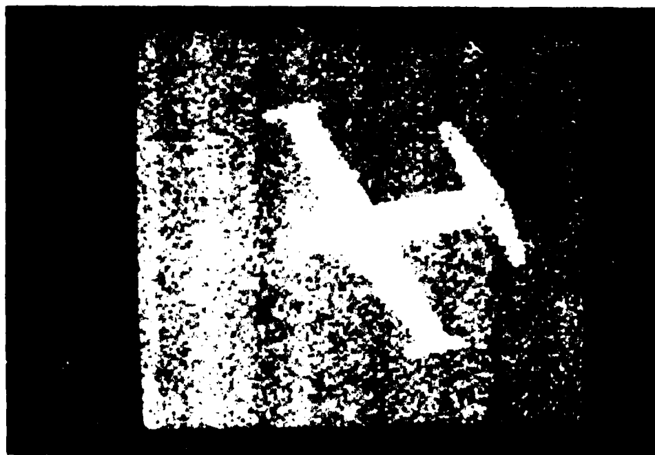
Figure 2.24 F104 image with noise added ( \text{SNR} = 10 \text{ dB} ), 128 \times 128 image resolution.
