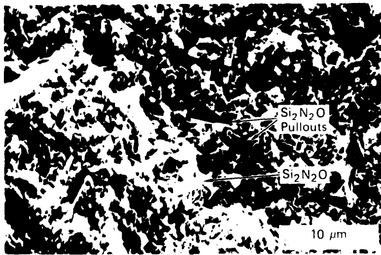
FIGURE 16 FRACTURE SURFACE IN A THICK JOINT Note pullouts and \text{Si}_2\text{N}_2\text{O} crystals.
