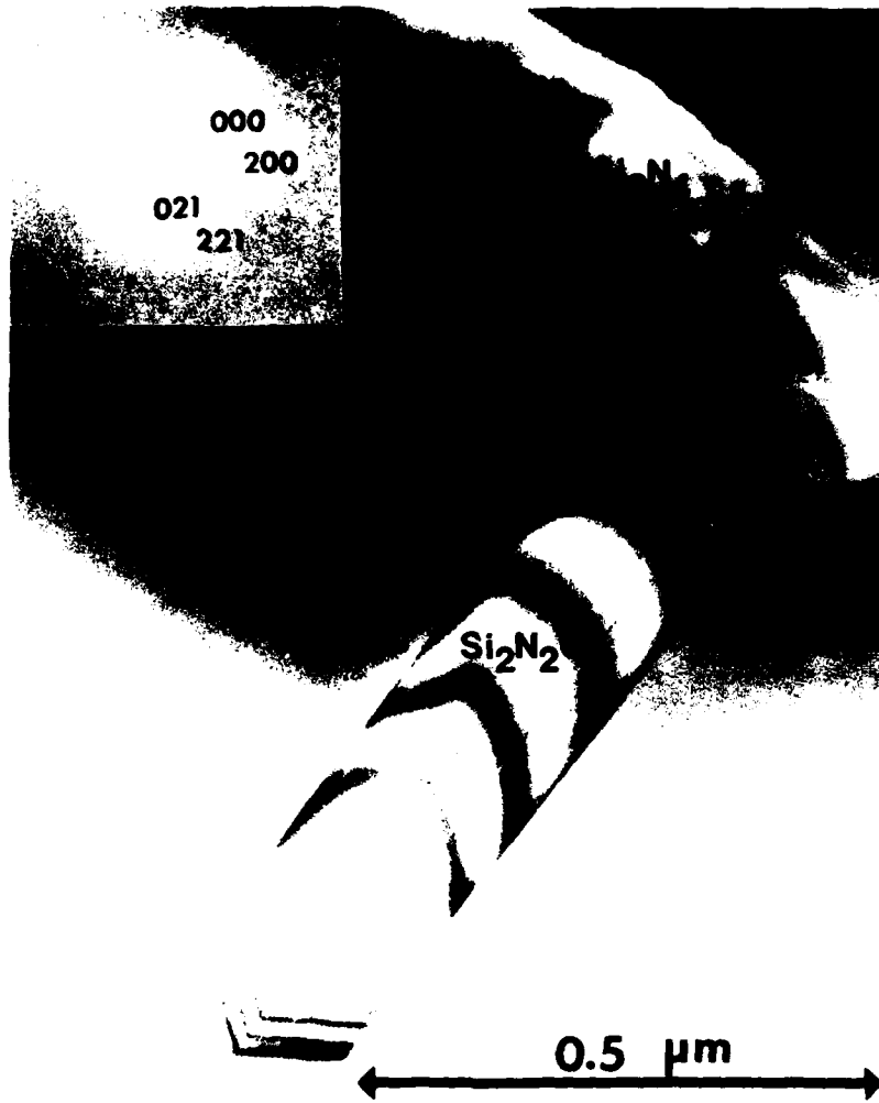
FIGURE 10 Si 2 N 2 O CRYSTAL GROWING INTO GLASS FROM AREA OF DISSOLVING SiN 4
