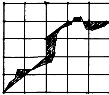
Figure 4-7 Overlay of Coded Line onto Input Line
